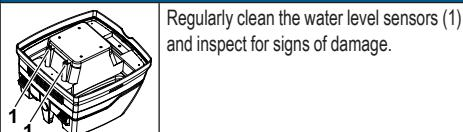
Regularly clean the water level sensors (1) and inspect for signs of damage.
