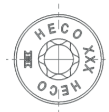
Head markings for d = 7.0 bis 12.0 mm all head types Head types without lettering possible.
