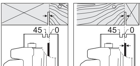
The  $0^\circ$  cutting mark **9** indicates the position of the saw blade for right-angled cuts. The  $45^\circ$  cutting mark **8** indicates the position of the saw blade for  $45^\circ$  cuts.
