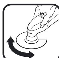
Work with low and uniform application pressure, otherwise, the working performance will decline and the application tool can become blocked.
