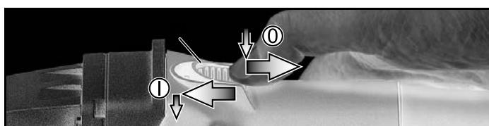
**Switching on/Continuous activation:** Push sliding switch (1) forward. For continuous activation, now tilt downwards until it engages.
